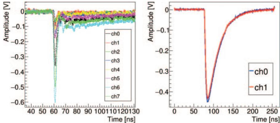
Fig. 4. – Example of the output signals of the SC (left), and of a single bar  $\Delta E$ -ToF (right), obtained with <sup>12</sup>C ion beam at 260 MeV/u. The two shown channels (ch0 and ch1) are collected at the two opposite extremities of the same bar.
