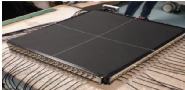
Fig. 2. – Picture of the  $\Delta E$ -ToF detector. The scintillator planes are enclosed in a black plastic cover that prevents the passage of light. The read-out channels, placed at the end of each bar, can be viewed.
