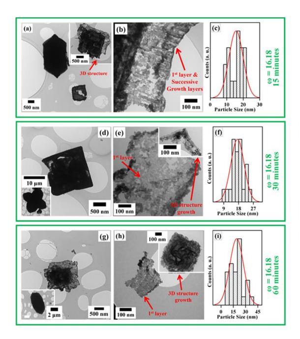
**Figure 4.** TEM images of samples "1" (a, b), "2" (d, e), and "3" (g, h); the histograms (c), (f) and (i) are the particle size distributions of the samples "1", "2", and "3" respectively; insets in (a), (e), and (h) are the layer by layer formed 3D structures of samples "1", "2", and "3", respectively. Insets in (d) and (g) are almond-like structures observed in samples "2" and "3" respectively.
