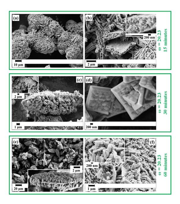
**Figure 3**. SEM images showing agglomerated truncated bi-pyramids of sample "4" (a), large almonds super-structures covered with sub-structures of samples "5" (c) and "6" (e), underdeveloped truncated bi-pyramids of samples "4" (b) and well organized through truncated facets truncated bi-pyramids of samples "5" (d) and "6" (f); inset in (b) shows magnification of rupture in truncated bi-pyramids of sample "4", in (e) magnification of a super-structure of
