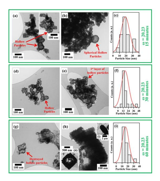
**Figure 5**. TEM images of samples "4" (a, b), "5" (d, e), and "6" (g, h); inset in (a) shows the successive layers of deshaped-hollow-spheres; insets in (h) show the cuboid and almond-like structures. The histograms (c), (f) and (i) are the particle size distributions of the samples "1", "2", and "3" respectively.
