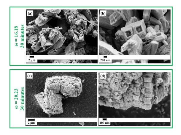
**Figure 10.** SEM images of dehydrated NiF<sub>2</sub> samples "2-2" (a, b), and "4-4" (c, d) prepared from the NiF<sub>2</sub>.4H<sub>2</sub>O samples "2" and "4", respectively, which were heated under vacuum at 250°C for 5 hours followed by heating under dynamic fluorine at 350°C for 5 hours.
