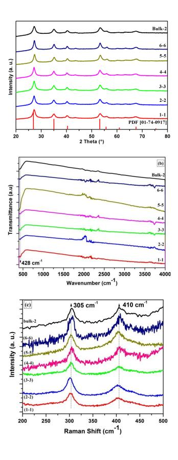
**Figure 8.** (a) Diffractograms, (b) FTIR, and (c) Raman spectra of NiF<sub>2</sub> samples "1-1", "2-2", "3-3", "4-4", "5-5" and "6-6" synthesized in a two-step process by the dehydration of NiF<sub>2</sub>.4H<sub>2</sub>O nanoparticles samples "1", "2", "3", "4", "5" and "6" respectively, and bulk NiF<sub>2</sub> ("Bulk-2") prepared from bulk NiF<sub>2</sub>.4H<sub>2</sub>O ("Bulk-1").
