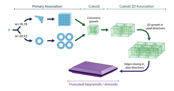
**Figure 6.** Schematic of cascade auto-organization process of nanoparticles/spheres into self-assembled super-structures
