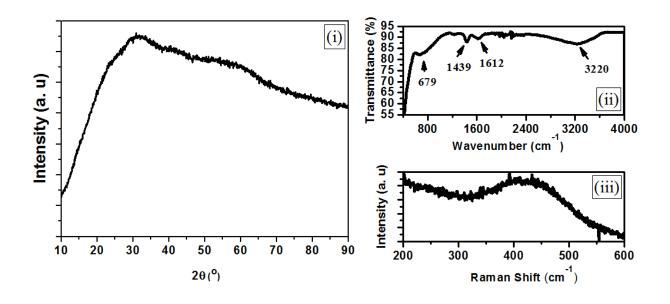
**Figure 7.** X-rays diffractogram (i), FTIR (ii) and Raman (iii) spectra of vacuum dehydrated NiF<sub>2</sub>.4H<sub>2</sub>O nanoparticles (sample 5) at 100°C for 1 hour followed by at 250°C for 5 hours.
