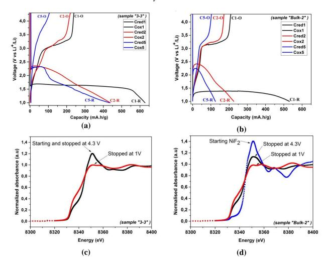
**Figure 11.** First, second and fifth galvanostatic cycles of half-cells using as cathode material sample "3-3" (a) compared to those of bulk material (*sample "bulk-2"*) (b). Oxidation and reduction process are labeled "Cox" and "Cred" respectively. XANES spectra of the nanostructured "3-3" (c) and bulk (*sample "bulk-2"*) (d) NiF<sub>2</sub> electrode materials before electrochemical measurements or after 1 full cycle and 1 reduction, stopped at 4.3 V or 1V.
