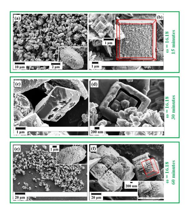
**Figure 2**. SEM images showing almond-like structures of samples "1" (a) and "3" (e), truncated bipyramids of samples "1" (b), "2" (c) and "3" (f), incomplete pyramidal wall encompassing auto-organized small pyramids of sample "2" (d), and auto-organized truncated bipyramids into superstructure of sample "3" (f); insets in (a) and (e) show magnified almond-like structures of samples "1" and "3", respectively
