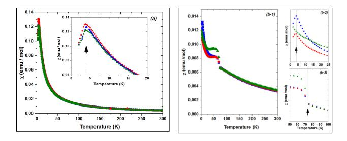
**Figure 12**. (a)  $\chi = f(T)$  curves for "bulk-1" (blue), sample "1" (red) and sample "6" (green), and (b) "bulk-2" (blue), sample "1-1" (red) and sample "6-6" (green) under a 5000 Oe dc magnetic field (zfc mode). Insert in figure (a) is a zoom around 4K for hydrated compounds, while figures (b-2) and (b-3) are zooms around 4K and 74K respectively for anhydrous compounds.
