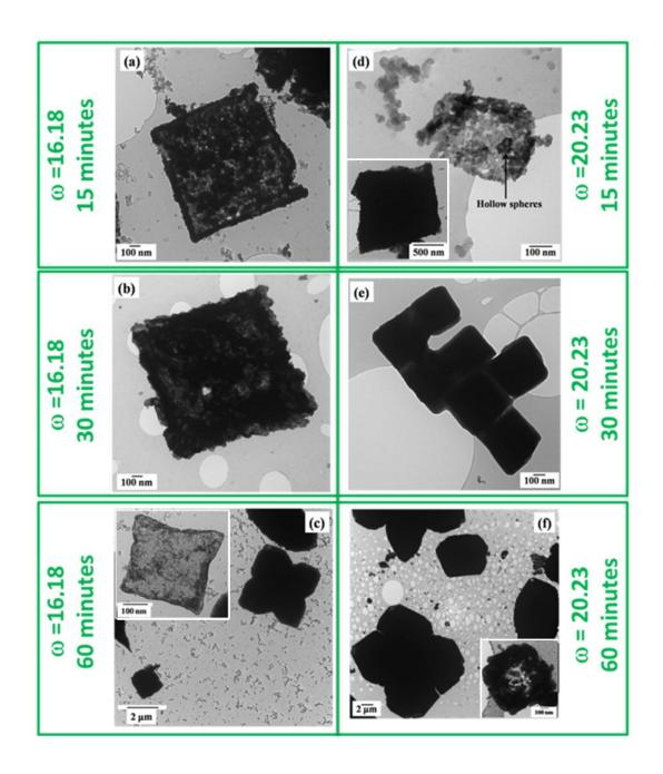
**Figure 9.** TEM images of samples "1-1" (a), "2-2" (b), "3-3" (c), "4-4" (d), "5-5" (e) and "6-6" (f) showing self-assembled nanoparticles giving cuboids and almond shaped super-structures; insets in (c) and (d) are shown the auto organized cubic structures in case of sample "3-3" and "4-4", respectively.
