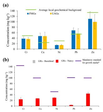
**Fig. 5** Bars plots of trace element concentrations (Cr, Cu, Cr, Ni, Pb, and Zn) in **a** urban allotment garden and former market gardens surface soils of Nantes (France) (green lines are the local geochemical background according to Le Guern et al. (2017) and **b** green roofs in Nancy. Purple continuous line represents the mandatory standard for growth media - Designations, specifications, marking - Supports de culture (\*) (AFNOR 2009)
