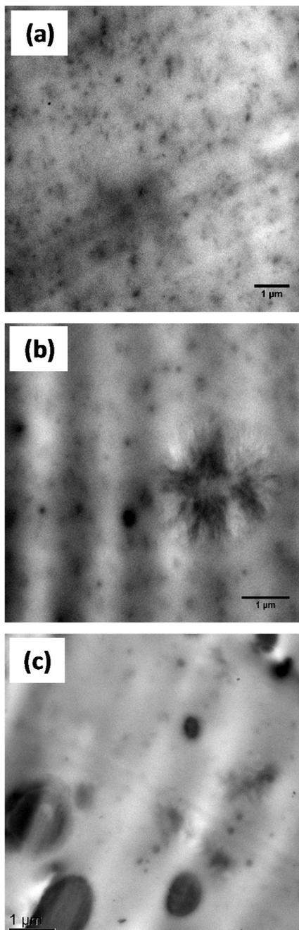
Figure S 2. TEM images of TPU containing MDI/BDO hard segments: a) 13wt% HS; b) 15wt% HS; c) 30wt% HS.
