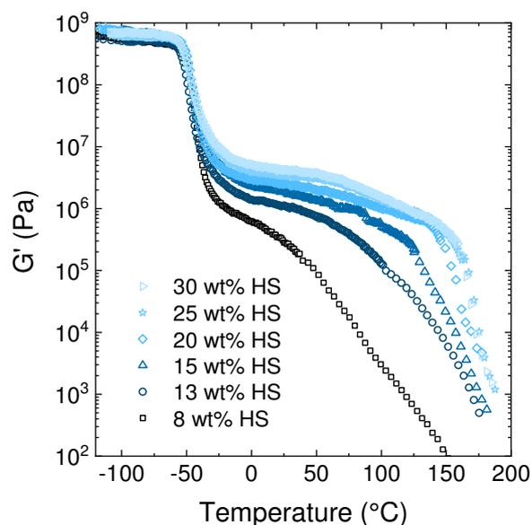
Figure 2. Storage shear modulus,  $G'$ , as a function of temperature at 1 Hz of TPU synthesized according to a two-step procedure and containing different amounts of MDI/BDO hard segment.
