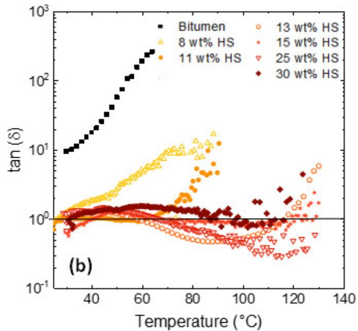
Figure S 6. Rheological properties of bitumens modified with 15 wt% of TPU at 1 Hz. Loss factor of blends containing TPUs with different HS contents as a function of temperature.
