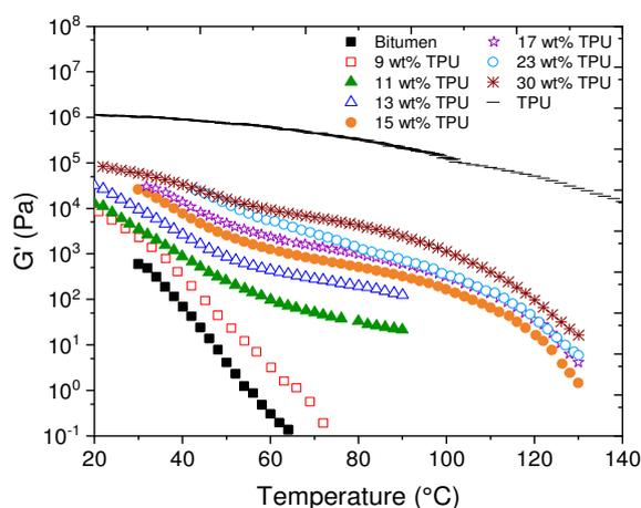
Figure 5. Rheological properties at 1 Hz of a bitumen modified with TPU13. Shear storage modulus of blends containing different TPU contents as a function of temperature.
