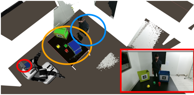
(a) The red circle indicates where the Kinect2 RGBD sensor is positioned, and the red rectangle indicates the camera view of the sensor. The orange circle indicates where interaction takes place, and the blue circle where the human is placed.
