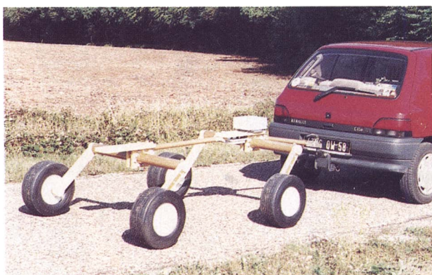
FIG. 2. Electrostatic quadripole designed for road studies where the poles are inside the tires of the wheels (1.2-m-side square array).
