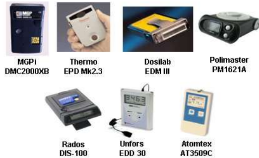
Figure 1. Active personal dosimeters tested in this study
