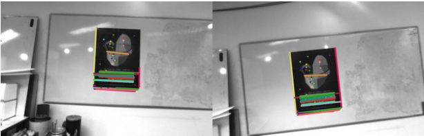
Fig. 3. Successful line matching between the image frame 169 (right) and the reference frame (left). Colorful points in both images are point correspondences used for our line matching algorithm.
