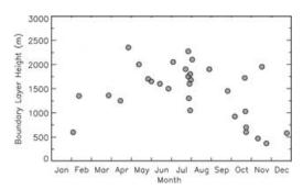
Fig. 4. Boundary layer height estimated from in-situ measurements of pressure, temperature, humidity, and CO<sub>2</sub>. Only mid-afternoon (12:00–17:00 LT) flights are considered.
