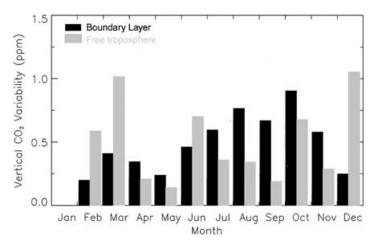
Fig. 6. CO<sub>2</sub> vertical variability within the boundary layer, and in the free troposphere as calculated from in-situ vertical profiles. The vertical variability is calculated as the standard deviation of residuals obtained after substracting for each vertical profile a smooth curve deduced from 50 m averaged data.
