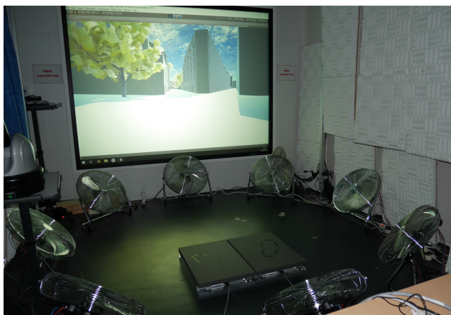
Figure 3: Location of the fans in front of the projection screen. Top image: fan layout around participants, units in meters. Lower picture: photography of the VR room.
