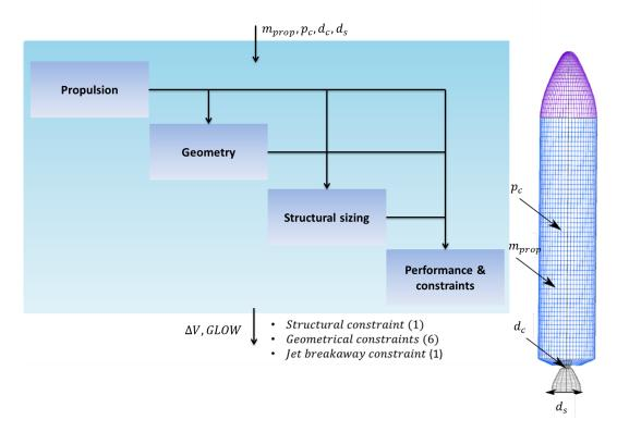
Figure 21: Optimization problem of a solid-propellant booster engine.
