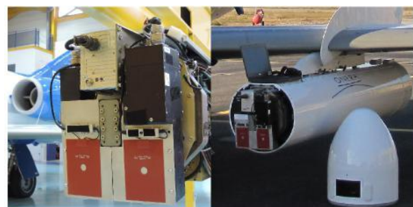
Figure 1 Camera VNIR1600 and SWIR256m-e inside the front part of the pod.
