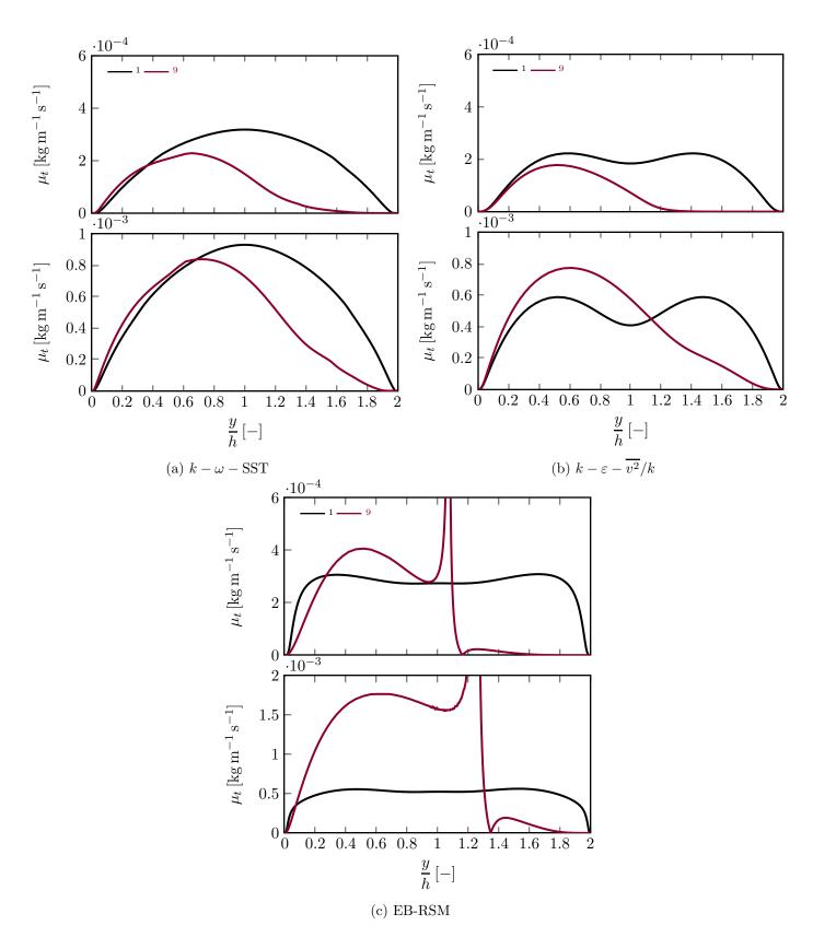
Figure 4 – Turbulent viscosity as a function of the non-dimensional distance to the cold wall for two temperature ratios ( $T_r = 1$  and 9) for the various RANS results for the lowest ( $\text{Re}_{\tau m} = 150$ , top) and highest ( $\text{Re}_{\tau m} = 375$ , bottom) turbulent Reynolds numbers
