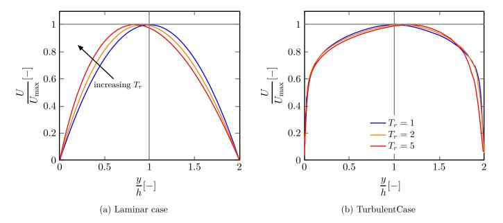
Figure 12 – Velocity profiles for non-isothermal Poiseuille flows
