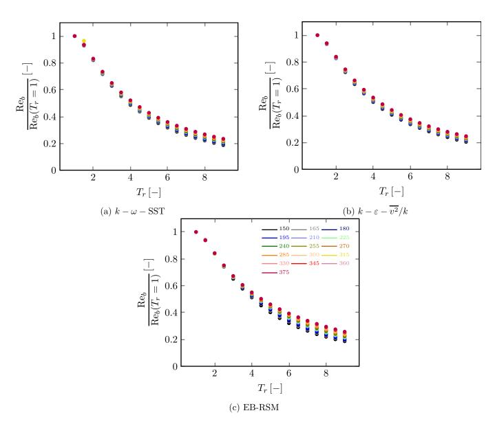
Figure 8 – Normalized bulk Reynolds number as a function of the temperature ratio for various turbulent Reynolds numbers
