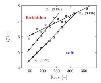
Figure 14 – Critical temperature ratio as a function of the turbulent Reynolds number for the three RANS models:  $k-\omega-{\rm SST}$  (triangle),  $k-\varepsilon-\overline{v^2}/k$  (circle), EB-RSM (square)
