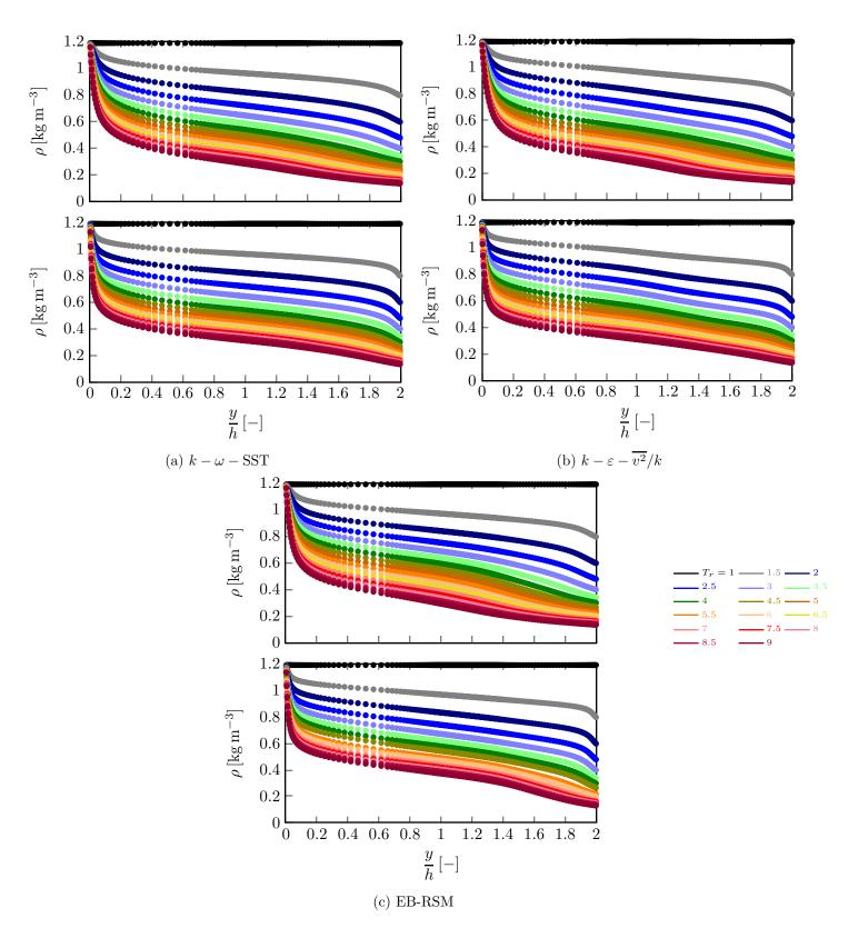
Figure 7 – Density as a function of the non-dimensional distance to the cold wall for the various temperature ratios for the lowest ( $\text{Re}_{\tau m} = 150$ , top) and highest ( $\text{Re}_{\tau m} = 375$ , bottom) turbulent Reynolds numbers
