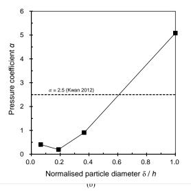
Fig. 2 (a) Influence of solid fraction on dynamic response of rigid barrier (redrawn from Song et al., 2017b) (b) Effects of particle size on dynamic response of rigid barrier (redrawn from Song et al., 2018)
