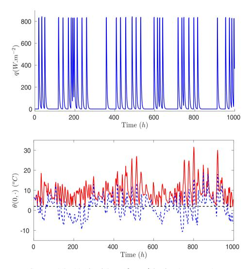
FIGURE 12. Source q defined by (5.14) for  $t \in [0, 1000]$  (Top) and corresponding temperature  $\theta(0, \cdot)$  at the road surface.
