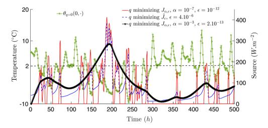
FIGURE 9. Surface temperature  $\theta_{q=0}(0,\cdot)$ , and sources q represented on [0,500] corresponding to the minimization of  $J_{\alpha,\epsilon}$  with  $\alpha=10^{-3}$  and  $\epsilon=2.10^{-13}$ ,  $\alpha=10^{-7}$  and  $\epsilon=10^{-12}$  and  $\tilde{J}_{\epsilon}$  with  $\epsilon=4.10^{-6}$ .
