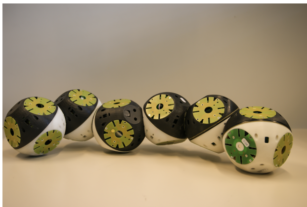
Figure 4: A snake-like formation of Roombot modular robots. (Courtesy of Prof Auke Jan Ijspeert, Biorobotics Laboratory, École Polytechnique Fédérale de Lausanne)
