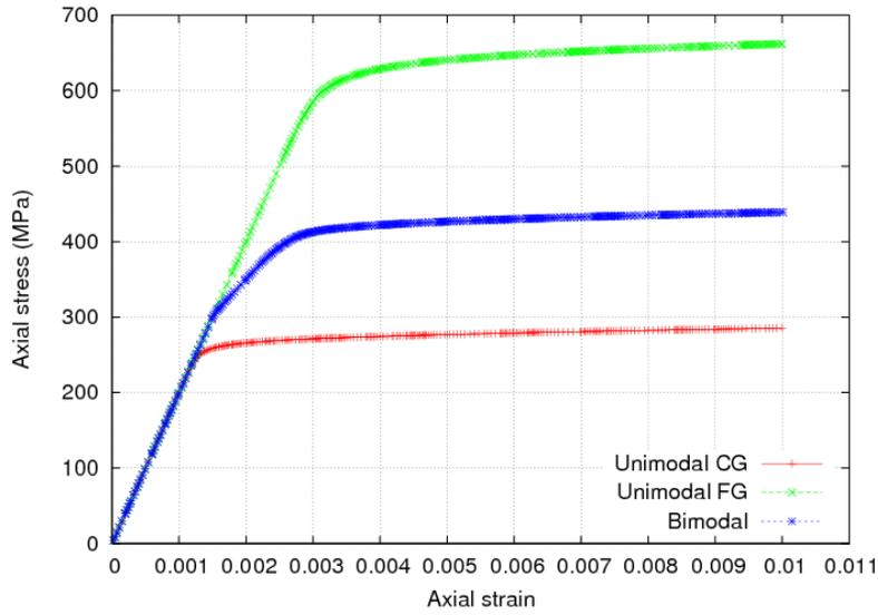
FIGURE 2: Tensile stress-strain curves of the three polycrystals.
