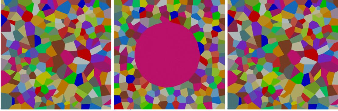
FIGURE 1: The three considered polycrystalline model microstructures. (From left to right) Unimodal Coarse Grain (grain size  $5\mu m$ ); Bimodal, with a single CG ( $5\mu m$ ) embedded in a matrix of FG ( $0.5\mu m$ ); Unimodal Fine Grain (grain size  $0.5\mu m$ ).
