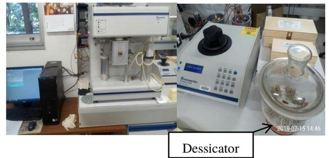
Figure 2. (a) Digital balance; (b) Gas displacement pycnometer with silicagel desiccator.
