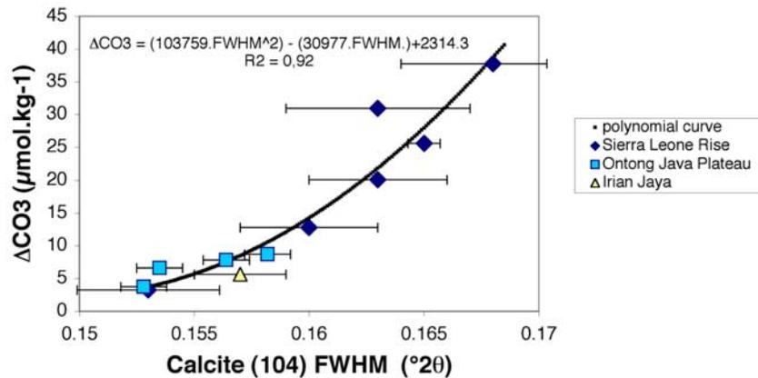
**Figure 4.**  $\Delta\text{CO}_3$  ( $=\text{CO}_3 - \text{CO}_{3\text{crit}}$ ) versus calcite (104) FWHM of *G. ruber*. Data from Sierra Leone Rise, Irian Jaya, and Ontong Java Plateau depth transects are plotted with a second-order polynomial regression curve. Standard deviations ( $1\sigma$ ) of data were calculated from six consecutive measures of the calcite (104) peak width from the same powder (see text for details). (Data from Ontong Java Plateau are from *Bonneau et al.* [1980].)
