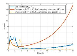
Fig. 1. Evolution of the  $\chi$ -norm of the closed-loop system with an input delay of 0.2s for three different strategies: a) Two actuators available, backstepping strategy [14], b) One actuator, naive backstepping strategy, c) One actuator, filtered control law (31).
