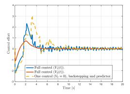
Fig. 2. Evolution of the control effort for two different strategies a) Two actuators available b) One actuator, filtered control law (31)
