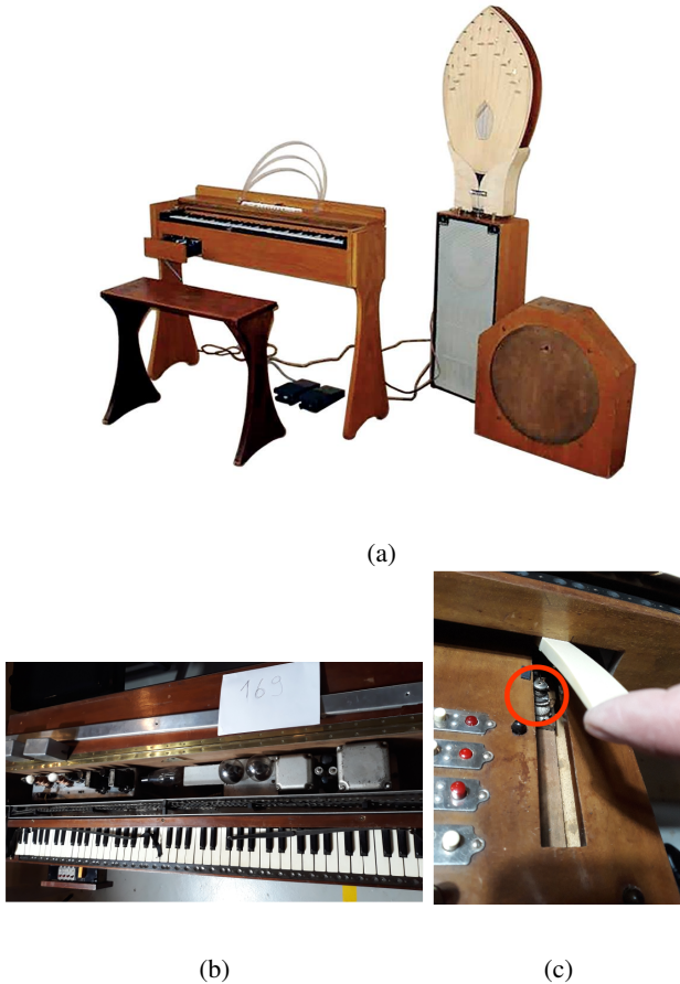
Fig. 1: Different parts of the ondes Martenot : diffuseurs (Fig. 1a on the right, from [33]), circuit, ribbon, keyboard (Fig. 1b), intensity key with the powder bag underneath circled in red (Fig. 1c).
