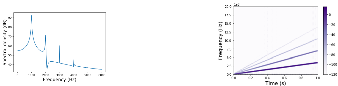
Fig. 11: Spectral density of the simulated power amplifier output voltage for an input of 1 kHz, amplitude 20 V.
