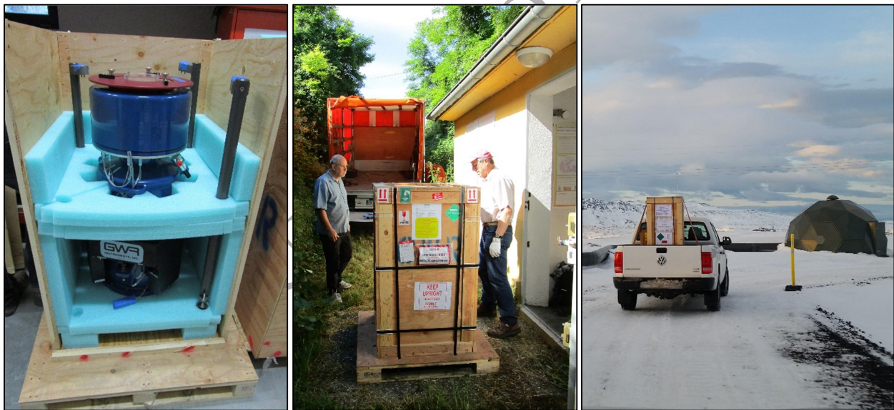
Figure A4. Packing and transport of the iGravs with liquid helium filled (4K, cold transport); after securing the Dewar and component parts inside the GWR supplied crates (a and b at J9, Strasbourg), the instruments were transported by truck and ship freight to the remote monitoring sites in Iceland (c).
