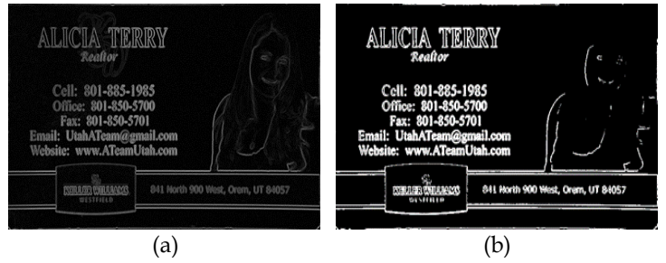
Fig. 4. Generation of binarized image (a) Morphological Gradient image (b) Binarized image.
