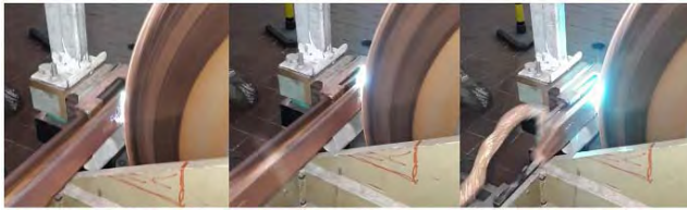
Fig. 5. Arc evolution on the wheel: ignition (left), elongation (middle), and quenching (right).
