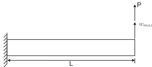
Figure 7.1: The cantilever straight beam.
