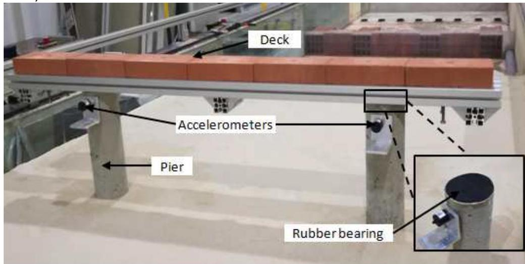
Figure 3: Experimental setup of the bridge configuration tests.
