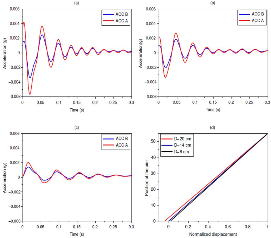
Figure 5: The filtered accelerations recorded with the accelerometer A and B (labels « ACC A » and « ACC B ») for the embedded lengths (a)  $D=20\text{cm}$ , (b)  $D=14\text{cm}$  and (c)  $D=8\text{cm}$  and (d) the corresponding modal shapes.
