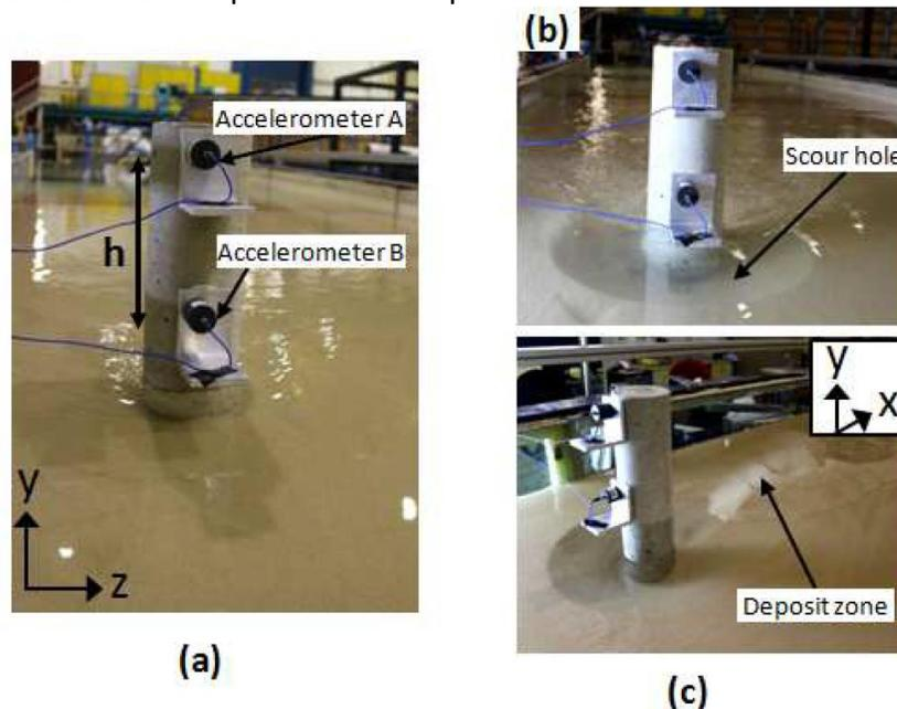
Figure 2: Experimental setup of single piers, water flume tests : (a) the initial configuration without scour ( $h$  the distance between the two accelerometers) (b) front view and (c) side view of the scoured configuration.
