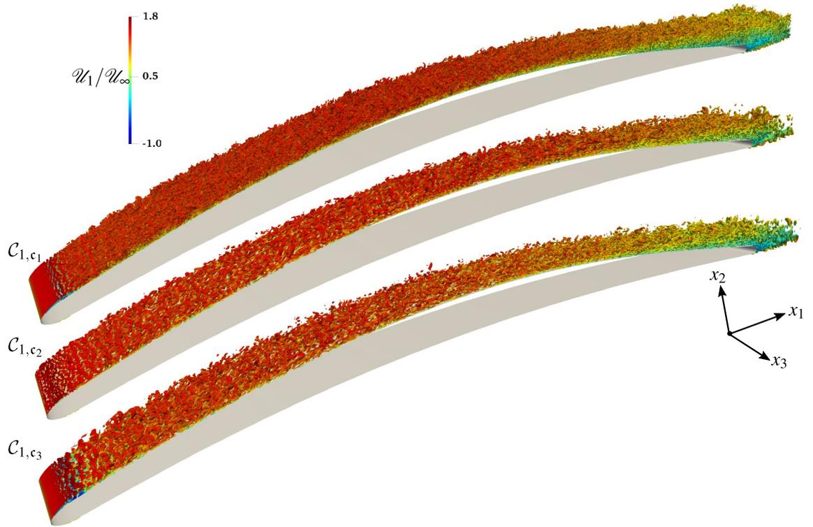
**Figure 4.** Topology of the flow described by the Q-criterion ( $Qc^2/U_\infty^2 \sim 950$ ) and colored by the normalized longitudinal instantaneous velocity  $U_1/U_\infty$  for the  $C_1$  cases for which  $Ma_\infty = 0.3$ ,  $Re = 8.30 \times 10^5$  and  $AoA = 4$ .
