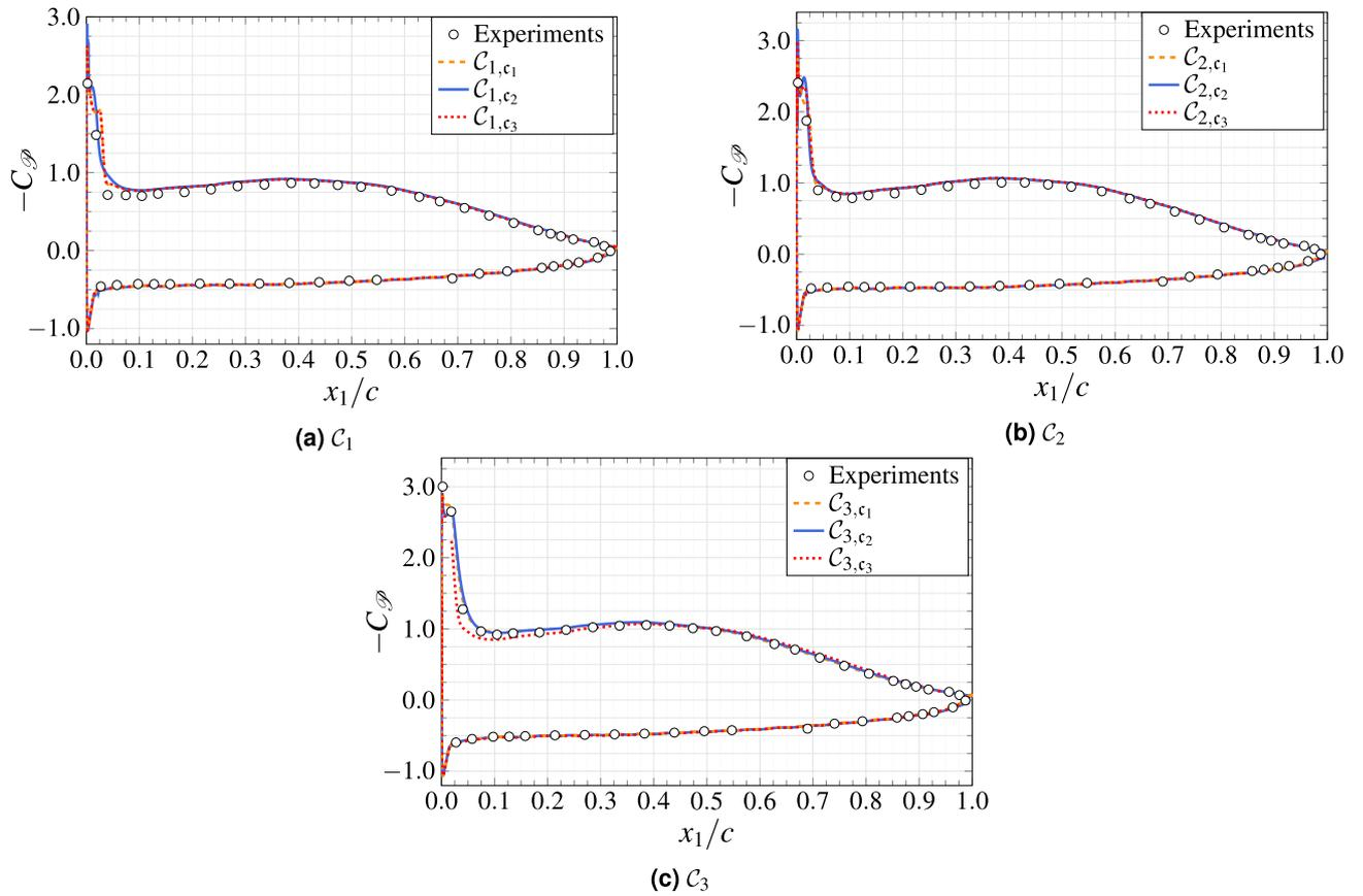
**Figure 7.** Comparison of the time-averaged pressure coefficient distribution.
