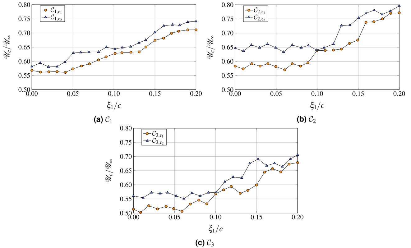
**Figure 16.** Convection velocity as a function of  $\xi_1$ , normalized by the chord. Reference probes used for the longitudinal spacing  $\xi_1$  is  $x_{ref} = 0.978$ .
