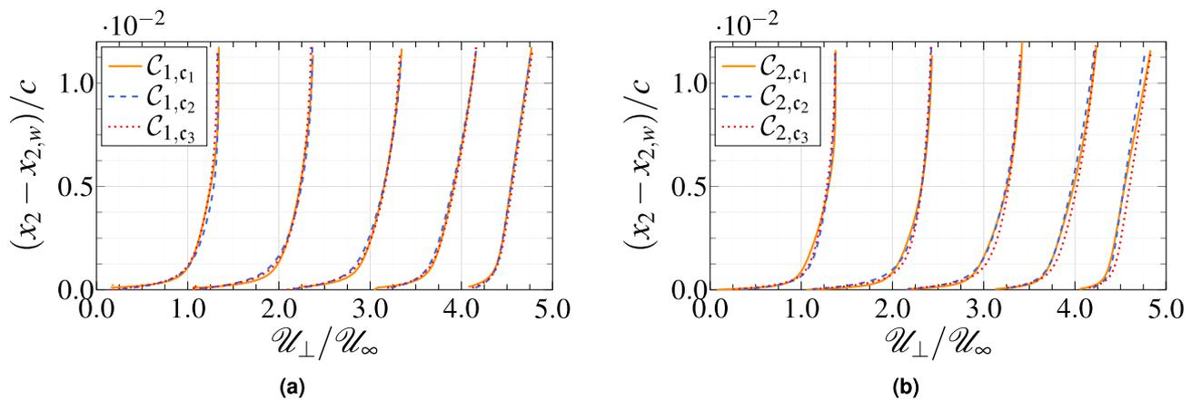
**Figure 8.** Mean streamwise velocity ( $U_{\perp}/U_{\infty}$ ) as a function of wall-normal distance at  $x_1/c = 0.1, 0.3, 0.5, 0.7$  and  $0.9$ . Each plot is separated by a horizontal offset of  $1.0$ .
