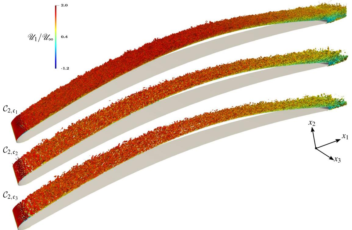
**Figure 5.** Topology of the flow described by the Q-criterion ( $Qc^2/U_\infty^2 \sim 950$ ) and colored by the normalized longitudinal instantaneous velocity  $U_1/U_\infty$  for the  $C_2$  cases for which  $Ma_\infty = 0.5$ ,  $Re = 2.29 \times 10^6$  and  $AoA = 4$ .
