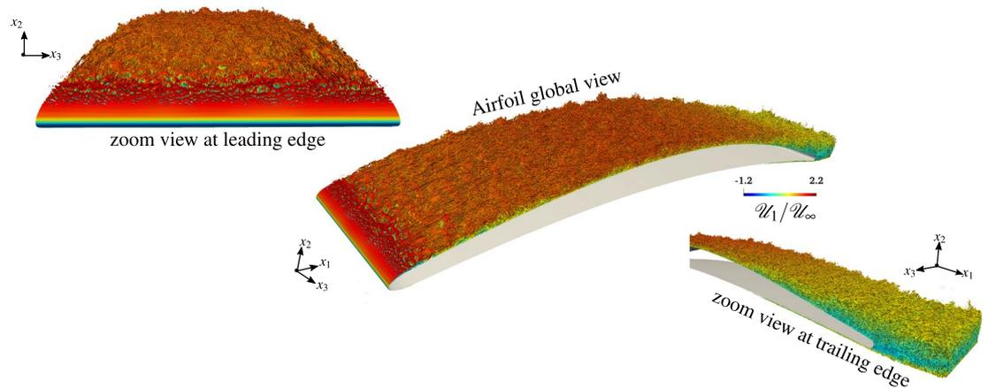
**Figure 3.** Topology of the flow described by the  $Q$ -criterion ( $Qc^2/U_\infty^2 \sim 950$ ) colored by the normalized longitudinal instantaneous velocity  $U_1/U_\infty$  for the  $C_{3,c_1}$  case for which  $Ma_\infty = 0.5$ ,  $Re = 2.29 \times 10^6$  and  $AoA = 5^\circ$ .
