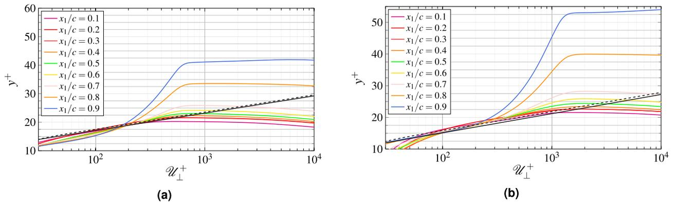
**Figure 10.** Profiles of the mean wall tangential velocity along wall-normal distance. The dashed line corresponds to the Reichardt law of the wall and the solid line to the classical law of the wall. The case  $C_3$  shows the same behavior and thus, for brevity, is not plotted.
