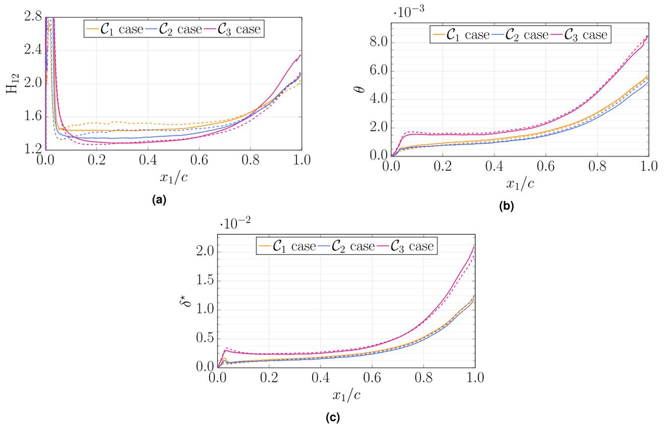
**Figure 11.** Variations of shape factor  $H_{12}$ , momentum thickness  $\theta$ , and displacement thickness  $\delta^*$  with chordwise distance  $x_1/c$  between WRLES computations (solid lines, cases  $\mathcal{C}_{*,c_1}$ ) and WMLES computations (dashed lines, cases  $\mathcal{C}_{*,c_2}$ ).
