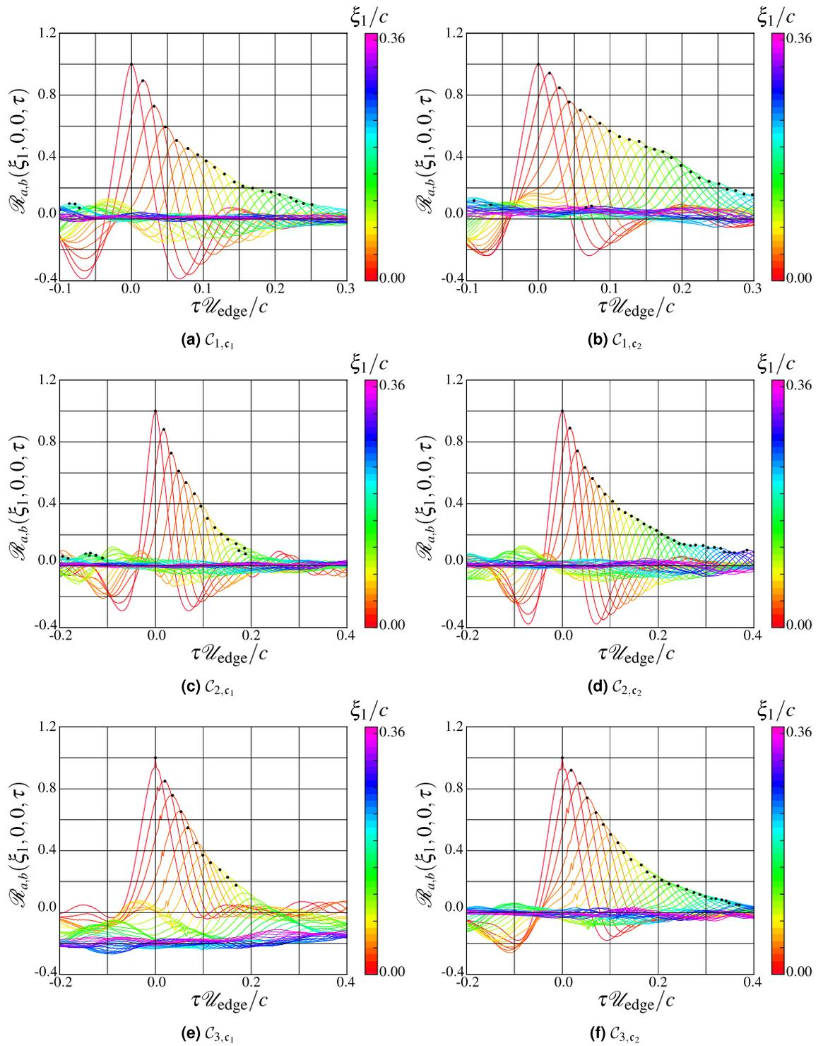
**Figure 15.** Cross-correlation functions of the simulated surface pressure fluctuations on the controlled-diffusion airfoil at suction side computed for different normalized streamwise separations  $\xi_1/c$ .
