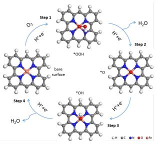
**Fig. 1** Schematic presentation of the four-electron mechanism for the electrochemical ORR. A limited H-terminated cluster model of the site is used and grey, blue, orange, red and white spheres represent C, N, Fe, O and H atoms, respectively.
