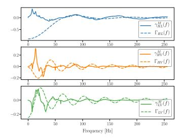
FIG. 3. From top to bottom we show  $\gamma_{ij}^M(f)$  (solid lines) and  $\Gamma_{ij}(f)$  (dashed lines) for ij = HL, HV, and LV. We discuss how we measure  $\gamma_{ii}^M(f)$  in the Appendix.
