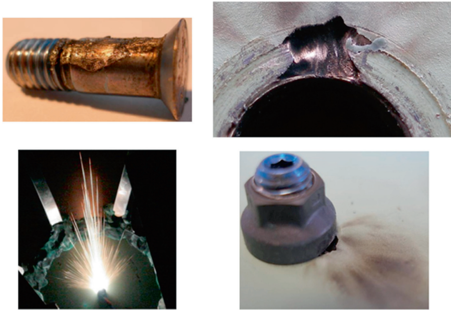
Fig. 1. Damage around the bolt fastener and ejected molten metal due to sparking.
