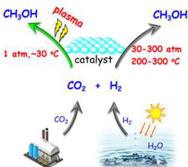
Figure 14. CO 2 hydrogenation to methanol using thermal catalysis and plasma catalysis. Reprinted with permission from [112]. Copyright (2018) American Chemical Society.
