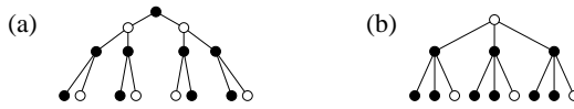
Fig. 6.12 Codewords are in black. (a) The complete binary tree of depth 4, with an optimal 1-LD code (of size 9) which is not 1-Id. (b) The complete ternary tree of depth 3, with an optimal 1-Id code (of size 9). This code is also an optimal 1-LD code.
