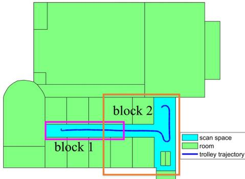
Figure 4. Trajectory of the trolley and blocks division.
