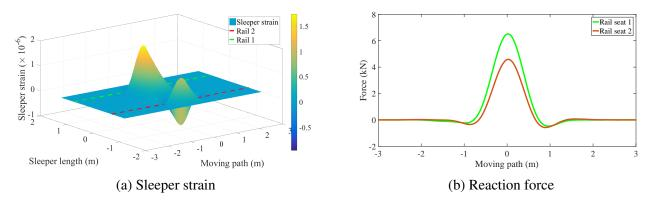
FIGURE 2 – Sleeper response under the lateral wheel loads
