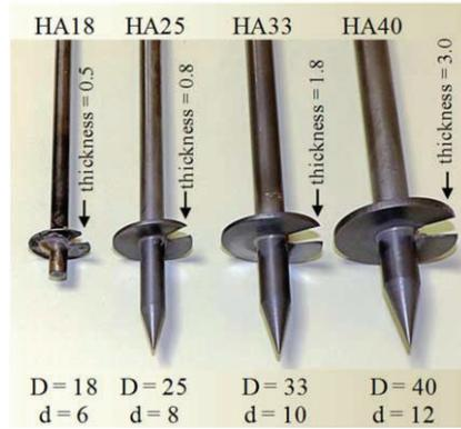
Figure 2. Helical anchor models (dimensions in mm).
