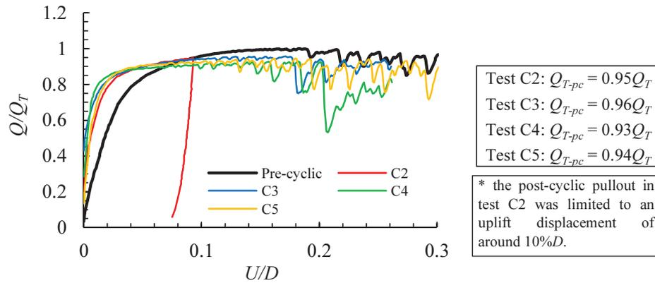
**Figure 6.** Pre-cyclic and post-cyclic monotonic load-displacement responses.
