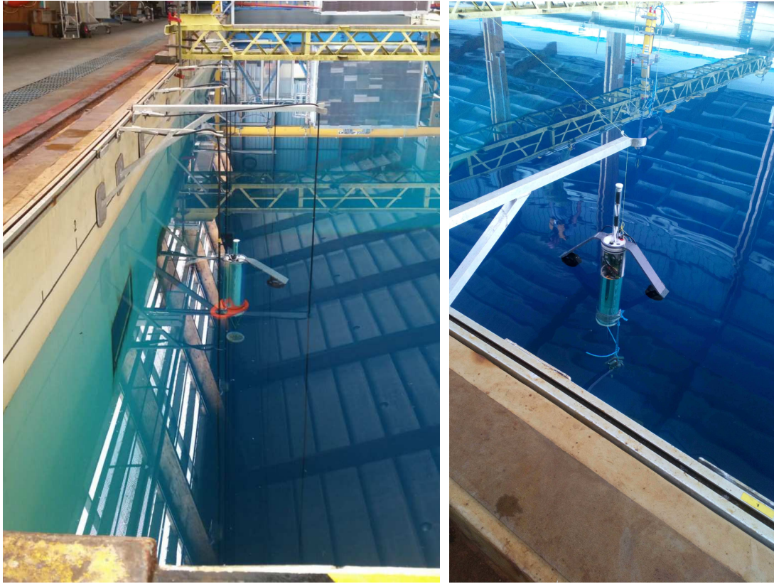
Fig. 9. Ifremer Brest water tank with the SeaBot float. The robot is secured along a rope guide.
