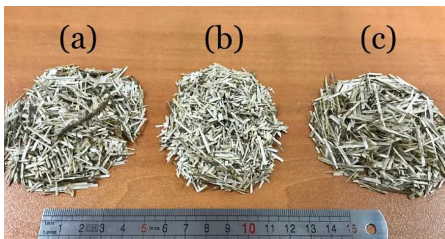
Figure 1. Photo of the flax shives used: (a) bulk size, (b) medium size, and (c) large size.
