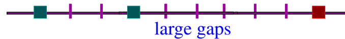
Fig. 3 fluid traffic: all cars are separated by large gaps, but in front of slow cars, the gaps are much larger.
