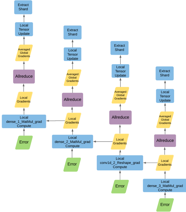
Fig. 3: Example execution graph augmentation: for each layer, the local gradient calculation for the lower layers can proceed in parallel with all-reduce and sharding
