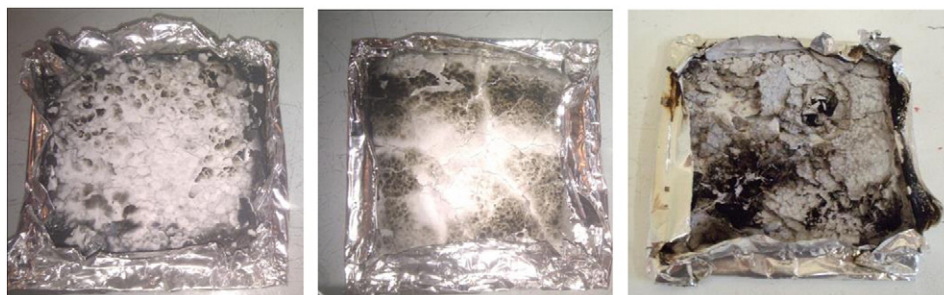
Fig. 9. Photographs of residues of PA6 composites: (left) K 1 PA, (middle) K 1A PA and (right) K 1E PA in the cone calorimeter test.
