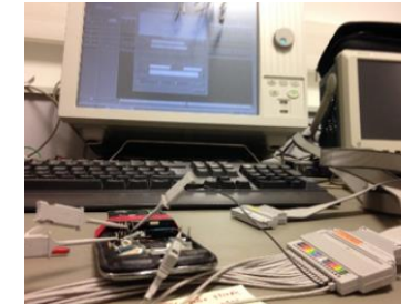
Figure 5: racking signals using a logic analyzer or an FPGA
