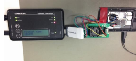
Figure 4: Reading operation under forensic bridge
