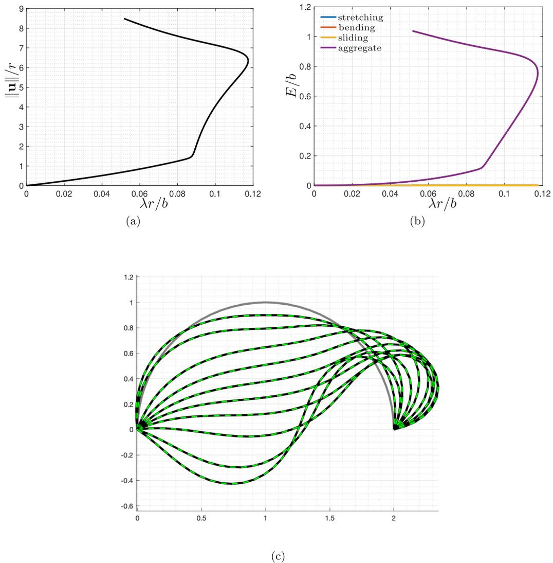
Fig. 20. Hinged semicircular arch with  $n = 36$  discrete elements. Equilibrium paths (a), energy evolution (b) and deformed configuration evolution (c) for  $a^2/b = 100000$  and  $cr^2/b = 100000$ .
