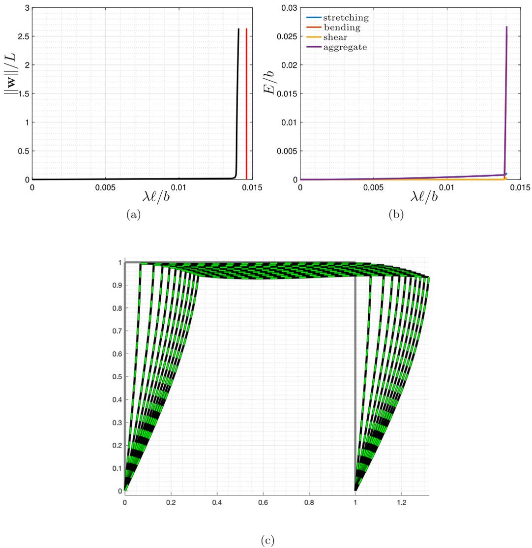
Fig. 14. Hinged-hinged frame made up of  $n = 48$  discrete elements. Equilibrium paths along with the reference solution for the buckling load in red color (a), energy evolution (b), and deformed configuration evolution (c) for  $aL^2/b = 1000$  and  $cL^2/b = 1000$  ( $\epsilon = 0.0001$ ).
