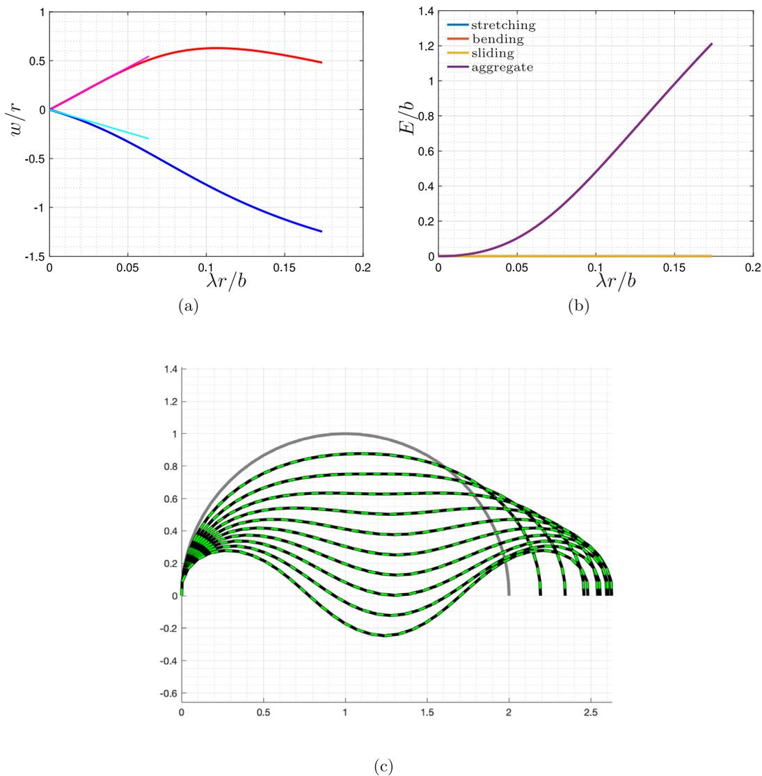
Fig. 16. Semicircular arch on sliders discretized with  $n = 36$  elements. Equilibrium paths (a), energy evolution (b), and deformed configuration evolution (c) for  $ar^2/b = 100000$  and  $cr^2/b = 100000$ .
