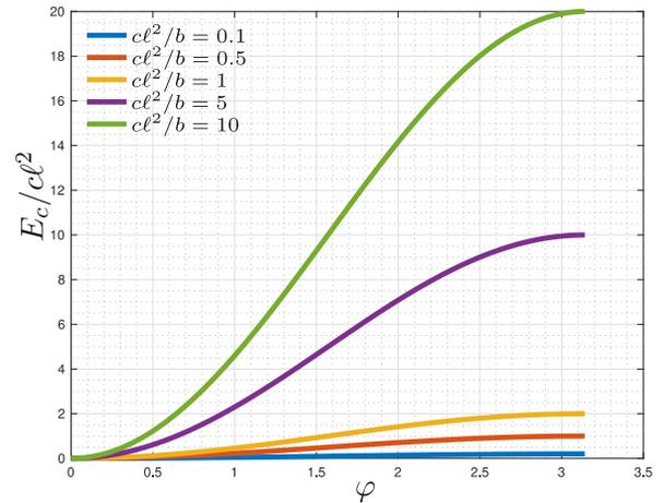
Fig. 5. Dimensionless shear strain energy  $E_c/cl^2$  versus  $\varphi$  for the third test as the non-dimensional stiffness ratio  $c^2/b$  varies from 0.1 to 10.
