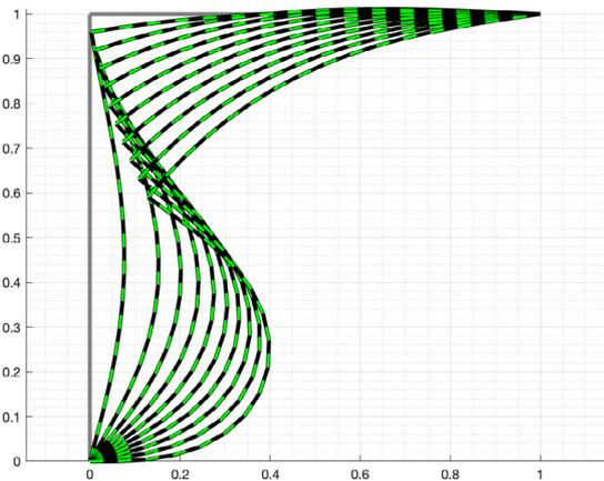
**Fig. 8.** Roorda's frame: evolution of deformed configuration for subsequent load steps ( $n = 32$ ,  $aL^2/b = 1000$ ,  $cL^2/b = 1000$ ,  $\varepsilon = 0.0001$ ).
