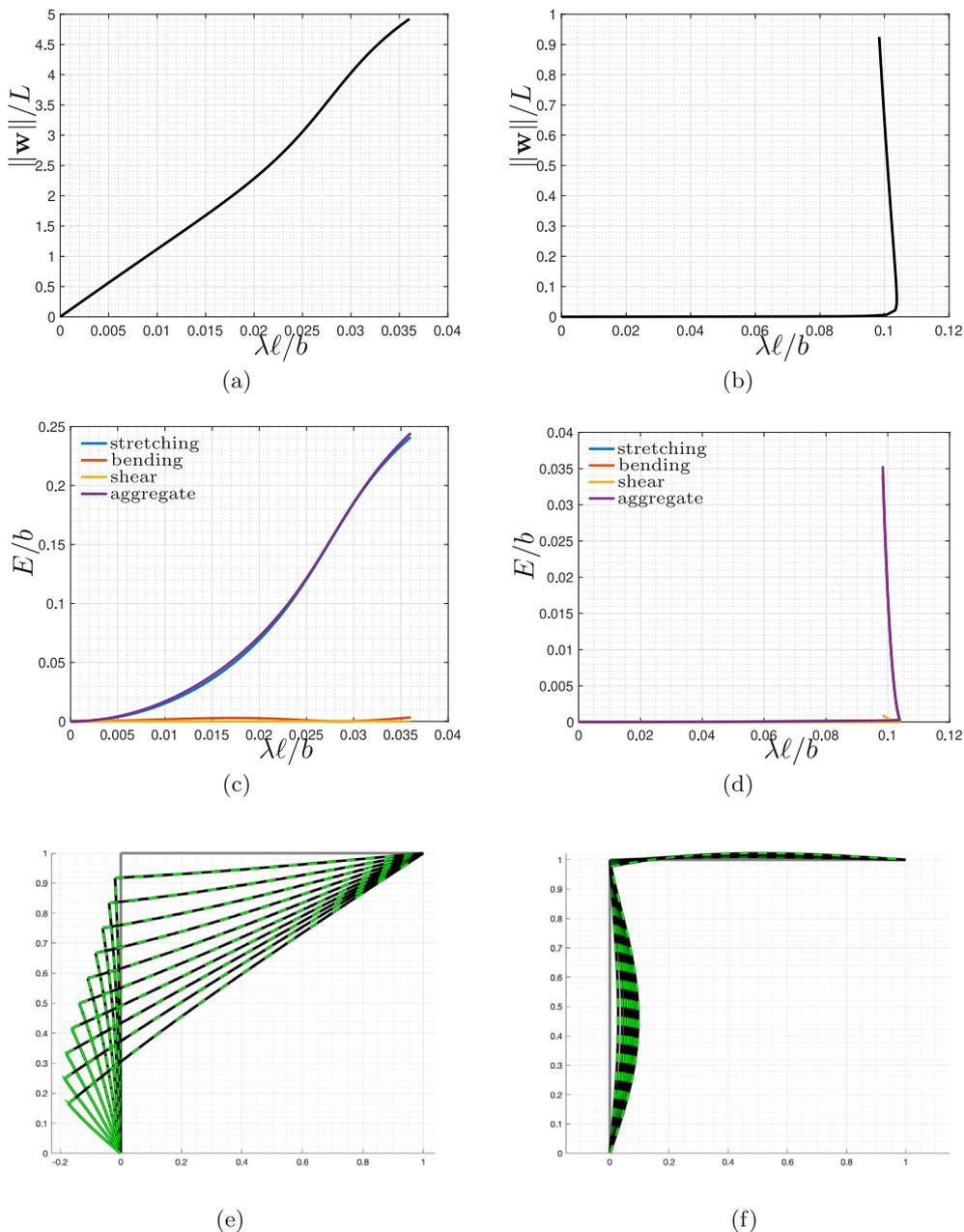
Fig. 11. Roorda's frame: results obtained by using  $n = 32$  discrete elements with  $aL^2/b = 10$ , on the left, and  $aL^2/b = 100000$ , on the right, ( $\epsilon = 0.0001$ ,  $cL^2/b = 1000$ ). Equilibrium path (1st row), evolution of non-dimensional strain energy contributions (2nd row) and of deformed configuration (3rd row) for subsequent load steps.
