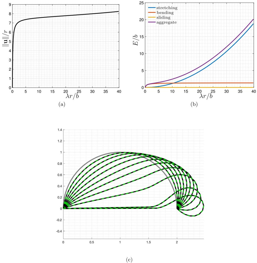
Fig. 19. Hinged semicircular arch with  $n = 36$  discrete elements. Equilibrium paths (a), energy evolution (b) and deformed configuration evolution (c) for  $a^2/b = 100000$  and  $c^2/b = 100000$  ( $\lambda_0 = 0$ ).
