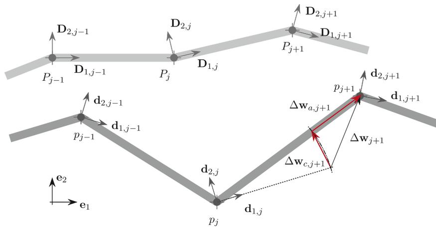
Fig. 1. Reference (light gray) and current (dark gray) configurations: stretch deformation  $\Delta w_{a,j+1}$  and shear deformation  $\Delta w_{c,j+1}$ , both in red color, for a Hencky-type discrete Timoshenko beam in plane.
