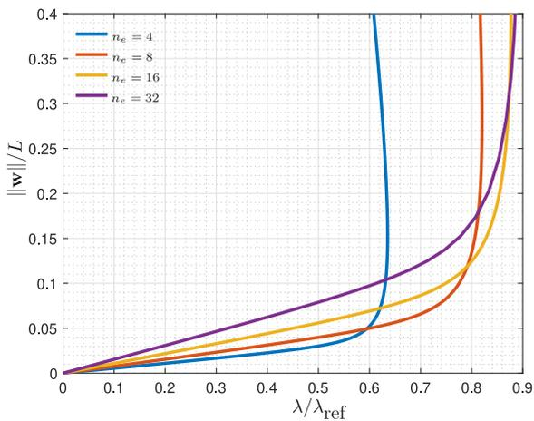
**Fig. 7.** Roorda's frame: equilibrium paths obtained by increasing the number of discrete elements  $n$  utilized to model the beams forming the frame ( $aL^2/b = 1000$ ,  $cL^2/b = 1000$  and  $\varepsilon = 0.0001$ ).
