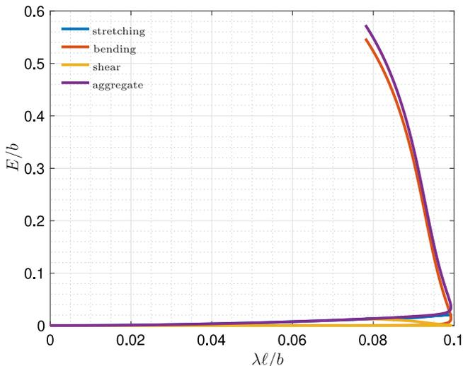
**Fig. 9.** Roorda's frame: dimensionless energy for subsequent load steps as split in stretch, bending and shear contributions ( $n_c = 32$ ,  $aL^2/b = 100$ ,  $cL^2/b = 1$ ,  $\varepsilon = 0.001$ ).
