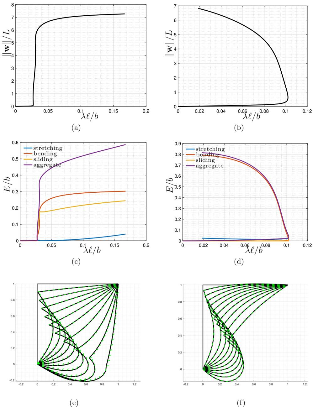
Fig. 12. Roorda's frame: results obtained by using  $n = 32$  discrete elements assuming  $cL^2/b = 10$ , on the left, and  $cL^2/b = 100000$ , on the right, ( $\epsilon = 0.0001$ ,  $aL^2/b = 1000$ ). Equilibrium path (1st row), evolution of non-dimensional strain energy contributions (2nd row) and of deformed configuration (3rd row) for subsequent load steps.
