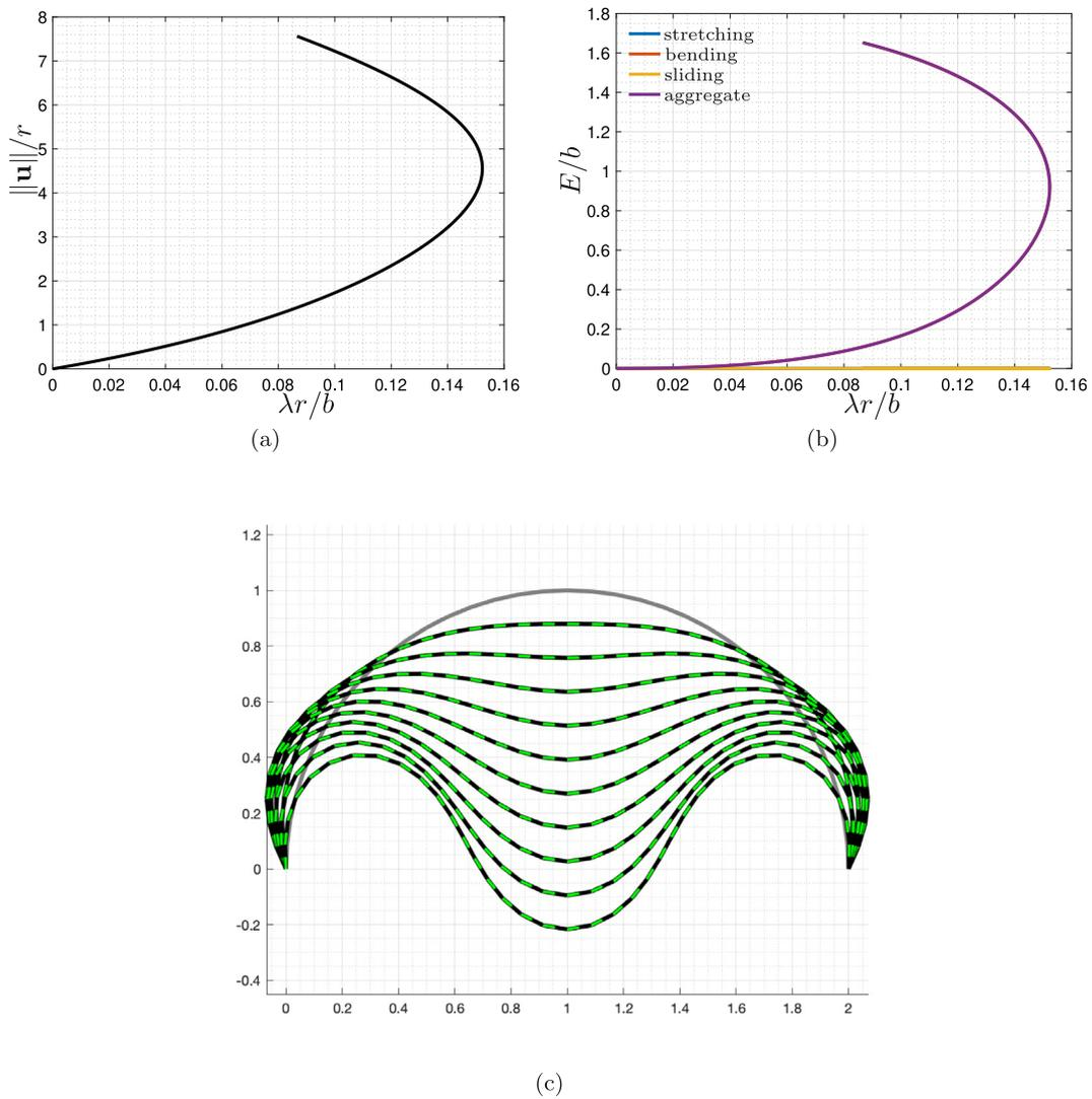
Fig. 18. Hinged semicircular arch modeled with  $n = 36$  elements: equilibrium paths (a), energy evolution (b) and deformation evolution (c) for  $a^2/b = 100000$  and  $c^2/b = 100000$  ( $\lambda_h = 0$ ).
