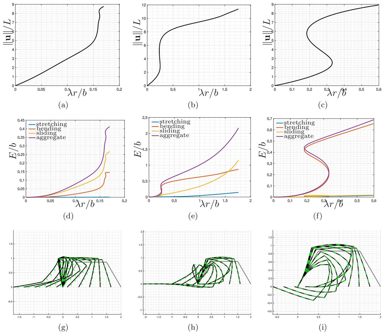
**Fig. 22.** Half regular hexagon cell with  $n = 15$  discrete elements. Equilibrium path (1st row), energy evolution (2nd row) and deformed configuration evolution (3rd row) for  $aL^2/b = 100$  and  $cL^2/b = 1$  (1st column),  $cL^2/b = 10$  (2nd column) and  $cL^2/b = 100$  (3rd column).
