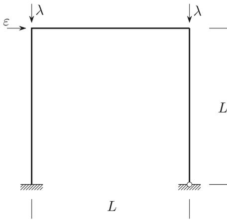
Fig. 13. Hinged-hinged frame under compression loads and horizontal imperfection load.
