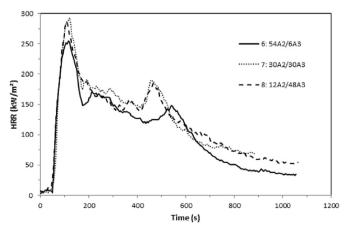
Fig. 8. HRR curves: Effect of bimodal mixtures SH100/SH20. 10%/90% (formulation 6), 50%/50% (formulation 7) and 80%/20% (formulation 8).
