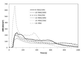
Fig. 9. HRR curves: Presence of silica-based fillers.
