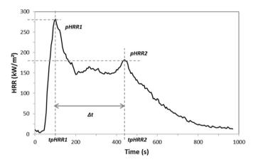
Fig. 1. A typical HRR curve with two peaks of heat release rate.
