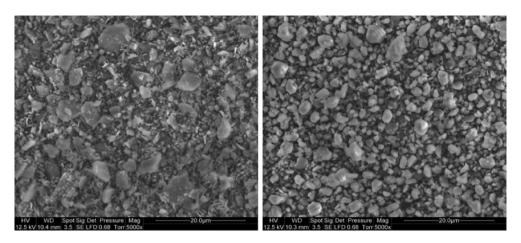
Fig. 7. Different shapes for ATH particles (left A4 - right A5).
