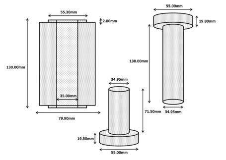
Fig. 2. A two-piston oedometric compression cell.
