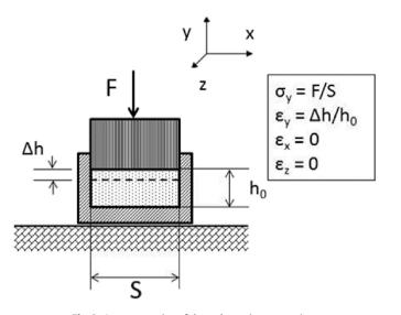
Fig. 3. A representation of the oedometric compression.
