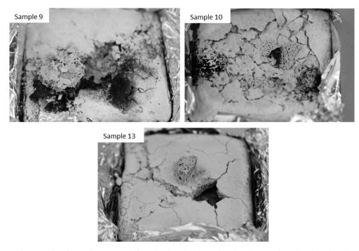
Fig. 10. Residue of cone calorimeter tests of sample 9 (50A2/10S1), sample 10 (50A2/10S3) and sample 13 (45A2/15S2).
