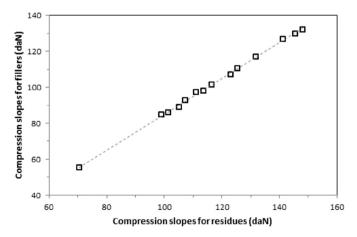
Fig. 14. Relation between slopes measured by oedometric compression for fillers and residues.
