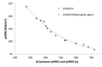
Fig. 11. Relation between the intensity of the second peak HRR and the duration between both pHRR.
