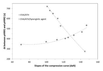
Fig. 13. Relations between the time to barrier layer breakdown during cone calorimeter tests and the slope of the compression curve for residue.
