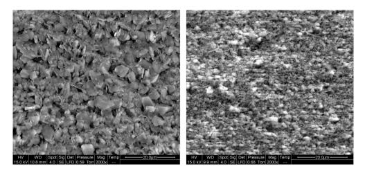
Fig. 12. Surface of the residue of formulation 3 (magnification: ×2000) and formulation 11 (magnification: ×2000).
