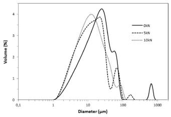
Fig. 5. Laser diffraction analysis of SH100 after different forces of compression (on fillers).
