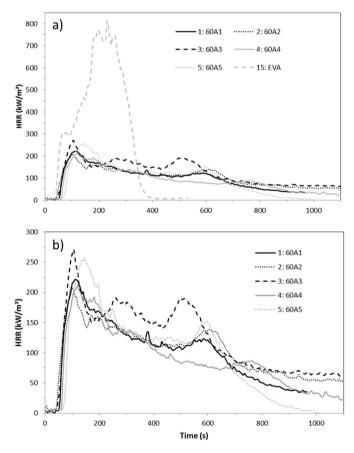
**Fig. 6.** HRR curves: Effect of different ATH (formulations 1 to 5) and comparison with pure EVA (formulation 15). All curves (a) and zoom without pure EVA (b).
