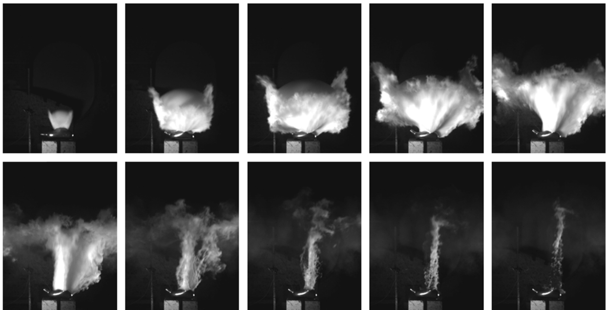
Fig. 8 – NTG Cylinder 2c=0.015 m, high pressure failure (44 MPa) with smooth dome ( \Delta t=0.28 ms).
