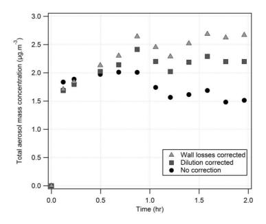
Figure 12 : Aerosol mass concentrations measured during the photocatalytic oxidation of ADOQ-50 emitted limonene in IRINA using Device 2 as a function of time, after dilution correction and wall losses correction ( $T = 22 \pm 1^{\circ}C$ ; RH = 50-60 %).
