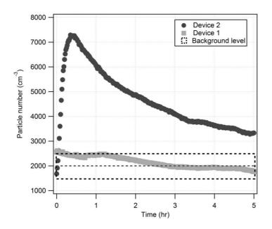
Figure 10 : Temporal evolutions of the number of particles during the treatment of household product emissions in IRINA using Device-1 and Device-2 ( $T = 22 \pm 1$  °C; RH = 50-60 %). The mean background level and the background variation zone are respectively marked with a dashed grey line and dashed black rectangle.
