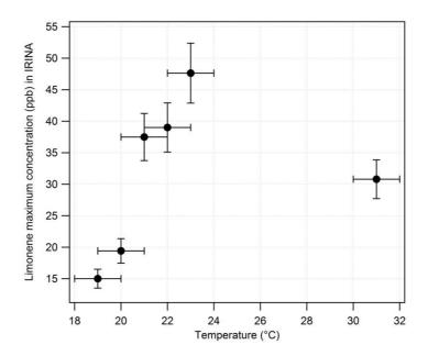
Figure 2: Evolution of limonene maximum concentration emitted from ADOQ-50 cleaning product as a function of the temperature set in IRINA experimental room (50-60 % RH). Error bars on x axis correspond to temperature standard deviation which is limited to  $\pm$  1 °C and error bars on y axis correspond to concentration measurement uncertainty which is determined as 10 %.
