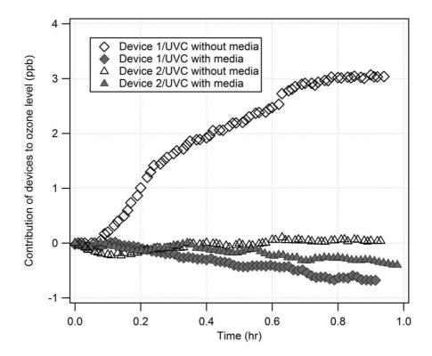
Figure 6: Evolution of ozone produced by Device-1 (diamond symbols) and Device-2 (triangle symbols) in IRINA experimental room as a function of time; t = 0 hr corresponds to the startup of devices; UVC lamps of devices are on, but devices are operated either with media (full symbols) or without media (empty symbols).
