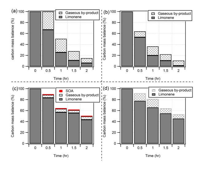
Figure 13: Respective contribution of limonene, identified gaseous reaction products and particulate matter into the carbon mass balance of VOCs emitted from household products using Device-1 ((a) at startup and (b) after 8h of operation) and Device-2 ((c) at startup and (d) after 8h of operation) (T°C= 22 ± 1°C; RH=50-60%).
