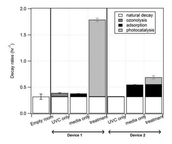
Figure 7: Decay rates of limonene determined in IRINA experimental room in the absence of any air treatment device (*empty room*) and in the presence of each selected device (*DEVICE-1* and *DEVICE-2*). Air treatment devices are operated (i) with UVC only and no media (*UVC only*), (ii) with media only and no UVC (*media only*) and (iii) with UVC irradiated media (*complete treatment*).
