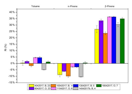
**Figure 6.** The canisters' response coefficient relative deviation from the NPL response coefficient. The legend displays the following information: the canister creation date (ddmmyyyy), the canister used (B denotes S053 and O denotes S052), and the number of replicates (n). Error bars show 1 standard deviation  $(1\sigma)$ .
