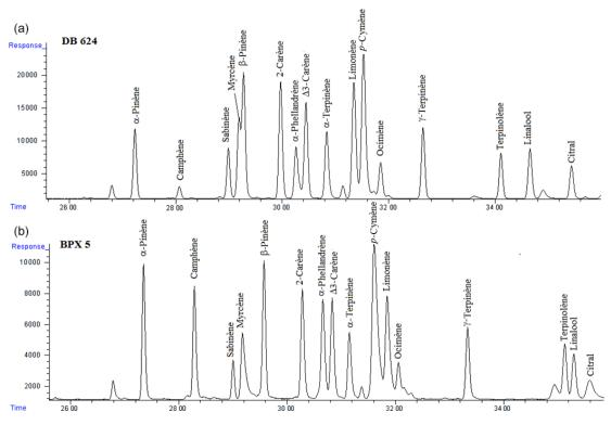
Figure 1. Separation of the 20 BVOCs from Table 2 using the DB-624 column (a) and the BPX5 column (b). VOC mixing ratios were approximately 1 ppb.
