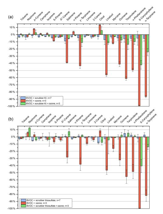
**Figure 5.** Relative deviation of BVOC measurements performed (i) with a scrubber and without  $O_3$ , (ii) when  $O_3$  (50 ppb) is added to the standard mixture without scrubber, and (iii) when a scrubber is used with  $O_3$ . (a) KI scrubber and (b) thiosulfate scrubber. VOCs are classified from the less reactive (left) to the most reactive (right) with ozone. Errors bars correspond to 3 standard deviations.
