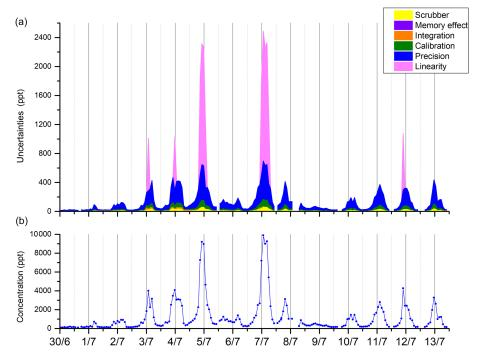
Figure 8. Repartitioning of uncertainties (k = 2) for the six terms considered (precision, calibration, integration, memory effect, scrubber, and linearity) (a) and the concentration of  $\beta$ -pinene during the LANDEX episode 1 field campaign (b).
