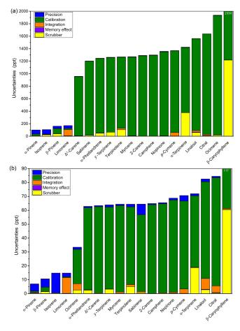
**Figure 7.** Repartitioning of uncertainties for the five terms considered (precision, calibration, integration, memory effect, and scrubber) at (a) 2 ppb and (b) 100 ppt with laboratory analytical parameters.
