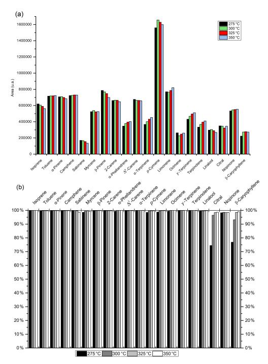
**Figure 3.** Investigation of the optimal desorption temperature for BVOC measurements. Two replicates performed at each temperature: (a) peak areas observed after the first desorption analysis and (b) the desorption efficiency.
