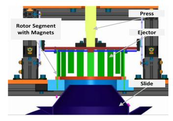
Fig. 3. Magnets dismantling concept of IPMSMs [7].
