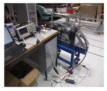
Fig. 9. Efficiency test bench with back-to-back configuration.
