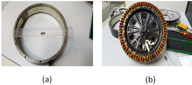
Fig. 8. (a) Outer rotor and magnets of the hub motor; (b) inner stator of the hub motor.
